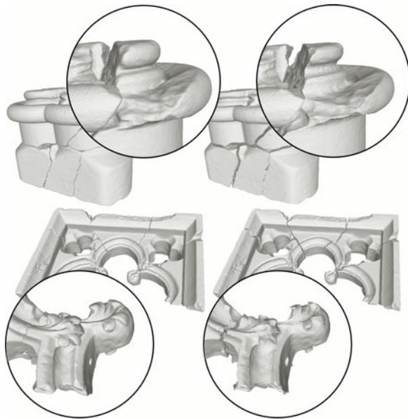
**Figure 7:** Two digitized and manually reassembled fragment sets made of limestone (top: column base, bottom: embrasure) before (left) and after (right) a simulation of 150 years of chemical weathering in polluted atmosphere.
