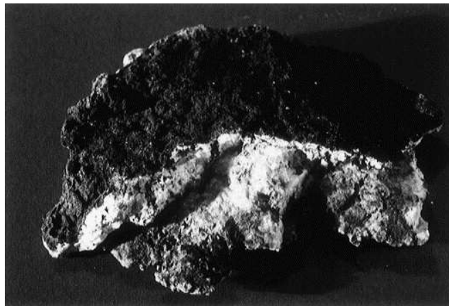
Figure 6: Stone from the Tiburtina Town Gate (Rome) showing the black crust due to atmospheric deposition. (Image from [39].)
