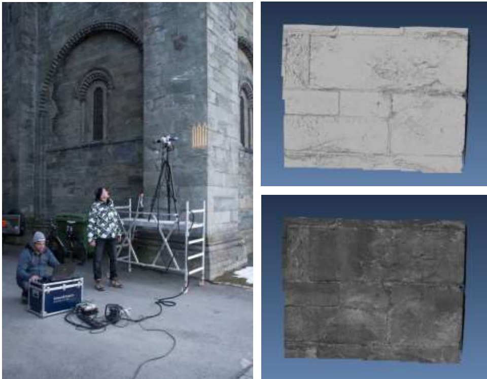
Figure 2. Scanning outside of the north entrance of Nidaros cathedral (left). The result from monochrome texture mapping (lower right image) using sensor imagery provides an added value for documentation and visualisation. (Images from 2013 campaign).
