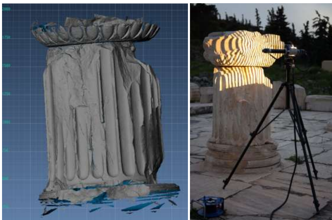
Figure 1. Visualisation of the 3D scanning results from Elefsis in OPTOCAT software (left, image from 2015 campaign). Data acquisition with a breuckmann Scanner (right, 2013 campaign).
